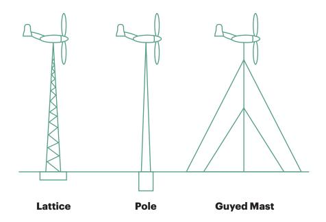
FIG. 1 Illustration of Various Types of Towers
